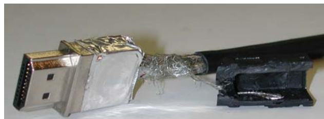
Figure 9. Poorly-shielded HDMI cable with only a few strands of braided shield contacting the metal tape on the plug.
