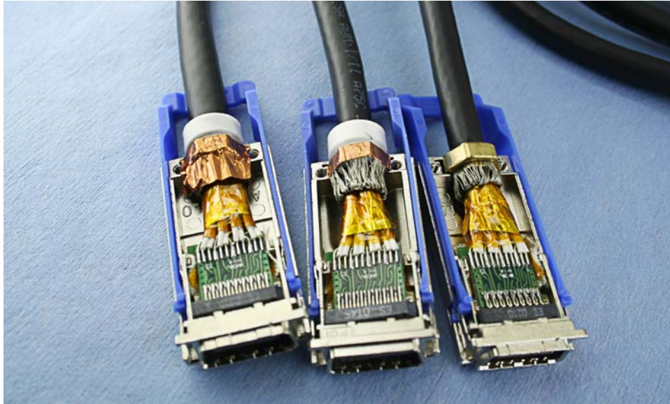
Figure 18. InfiniBand cable assemblies with different termination methods.
