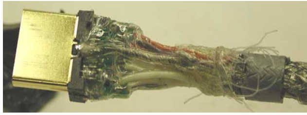
Figure 10. Poorly-shielded HDMI cable with cable braid stripped back and then attached to plug shell at only one point with a twisted pigtail.
