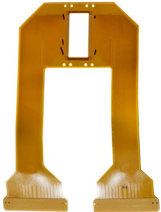
Figure 7: Stiffeners supporting SMT connectors and wire bond area.
