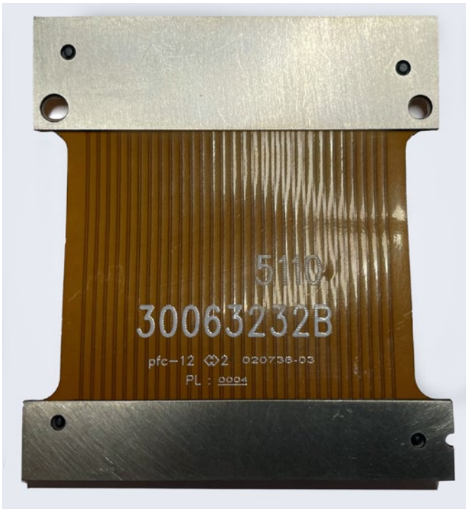
Figure 4: Stainless stiffener for flatness.
