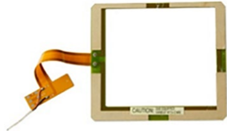
Figure 6: Stiffener supporting display.
