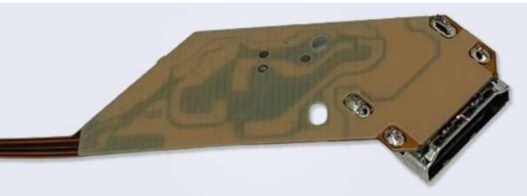
Figure 1: Mechanical support for SMT connector.
