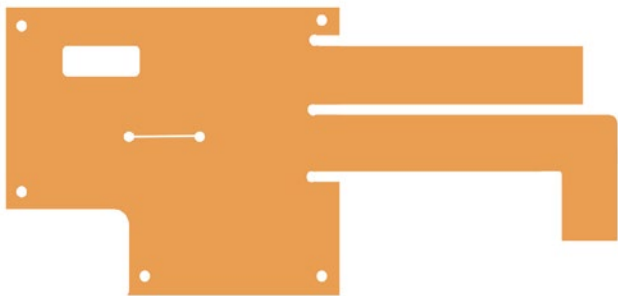
Figure 1: Flexible circuit outline example.
