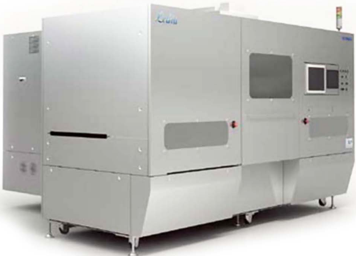
Figure 3: Ledia 5 Multiwavelength UV-LED direct imager.
