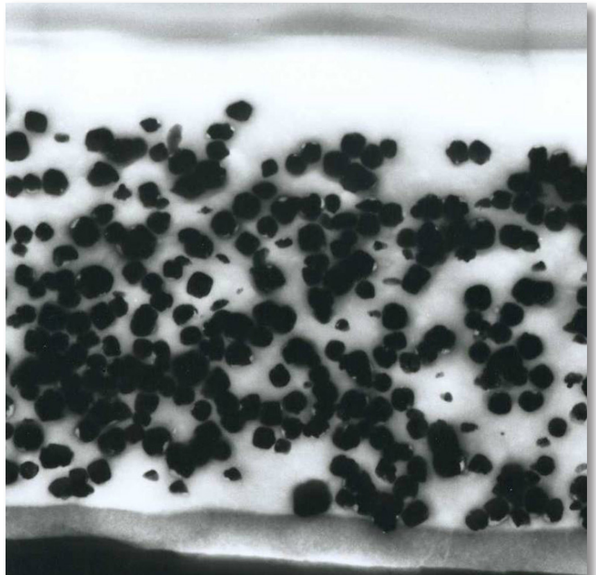
Figure 2: Cross-section of emulsion layer.
