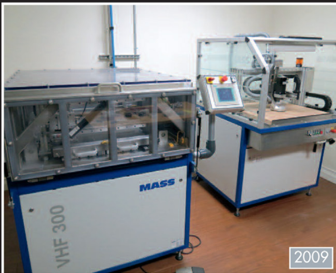
Mass VHF300 Via Fill Machine & SV100 Planarizer
