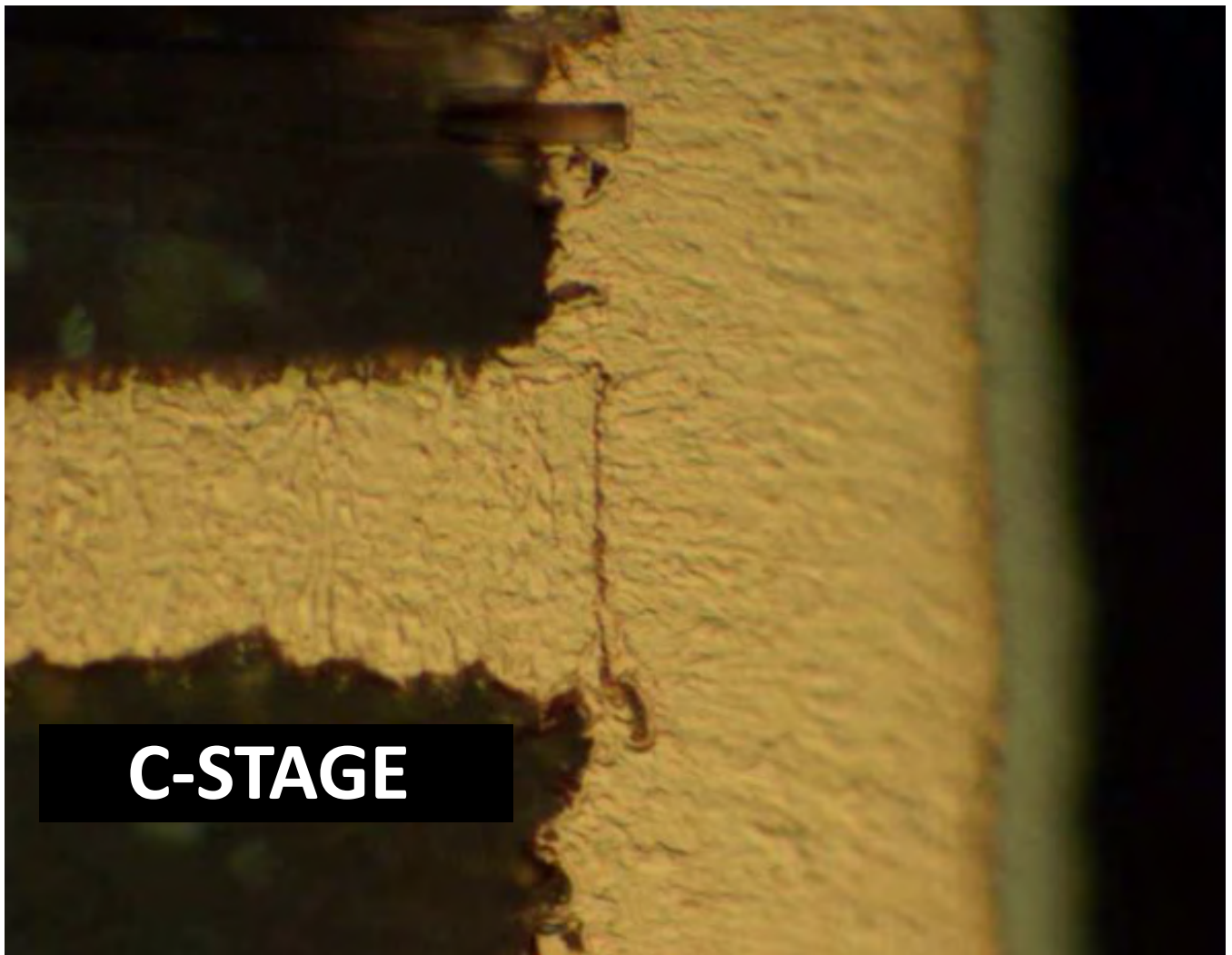
Figure 3: Zinc tail evident on C-stage.
