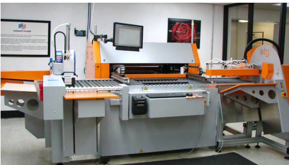
Figure 3: Colonial's newest electrical tester, an atg A7a, utilizes eight flying probe test heads for a wide variety of advanced, high-speed electrical test techniques, with an auto-load/unload system for true "lights-out testing."
