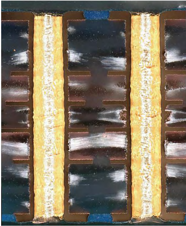
Figure 1: Cross-section of two vias with a measurable short showing CAF shorting in a layer of resin starved prepreg
