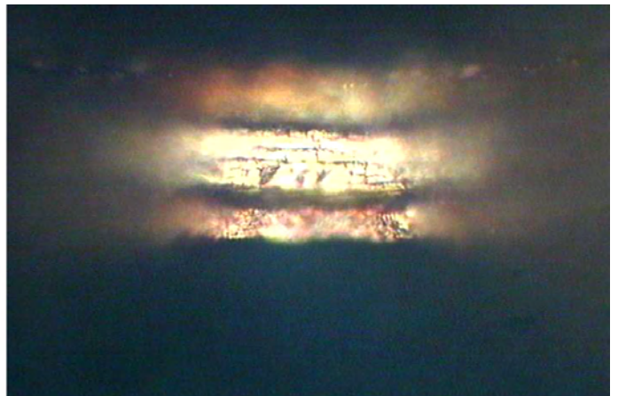
Figure 3: Dark area indicates no copper plating. This is a front light of the blind via.
