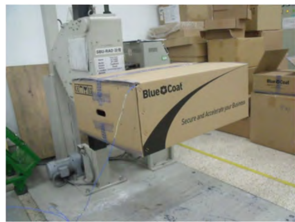
Figure 9: A shock gravitational force measurement device embedded in the shipping box.
