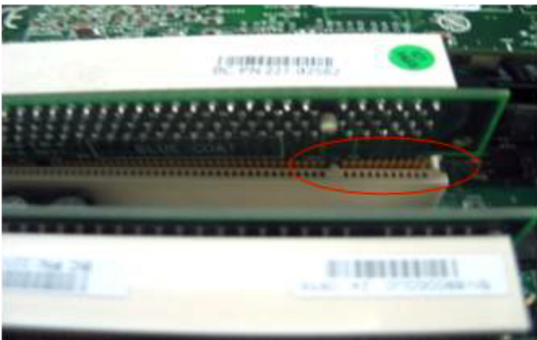
Figure 1: Example of partial loose contact of a daughter card from a press-fit connector.
