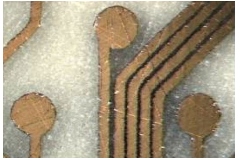
Figure 5: Traces, vias, and pads from Figure 4 now metallized and plated 2 .
