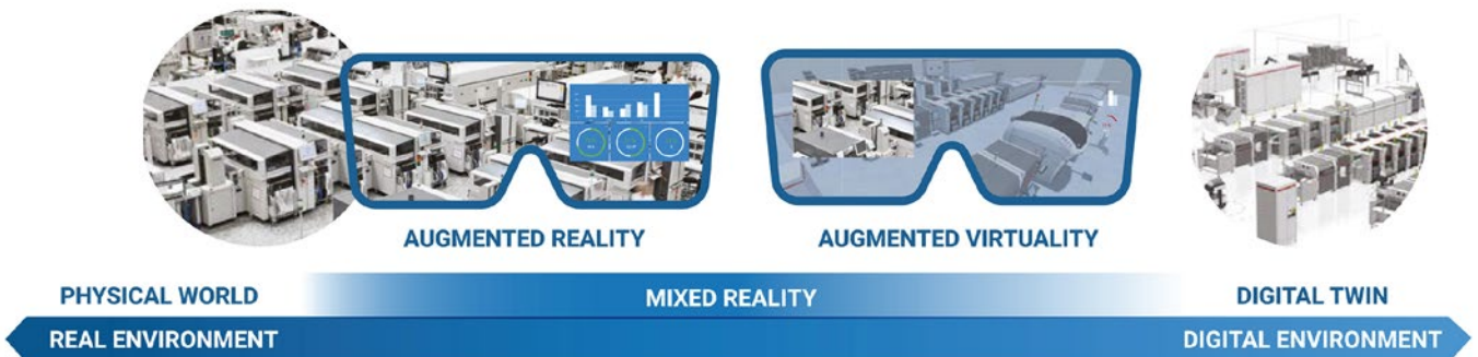
Figure 2: The reality-virtuality continuum includes not only real and virtual at each end, but also mixed reality. Mixed reality includes augmented reality (AR) where virtual elements are superimposed on a camera view of reality, and augmented reality, where views of reality are projected onto the virtual environment of a digital twin.
