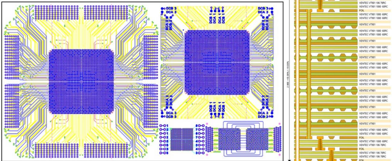
Figure 2: BGA coupon with real and daisy-chain component fanout for 1.0-mm and 0.8-mm pitch component (left) and build-up of the qualification test vehicle (right).
