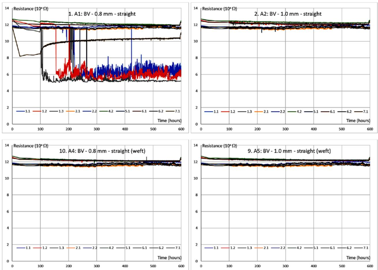
Figure 5: CAF test results for buried vias in a straight configuration with a pitch of 0.8 mm (left) and 1.0 mm (right) for both the warp (upper row) and weft direction (bottom row) of the glass fibers.
