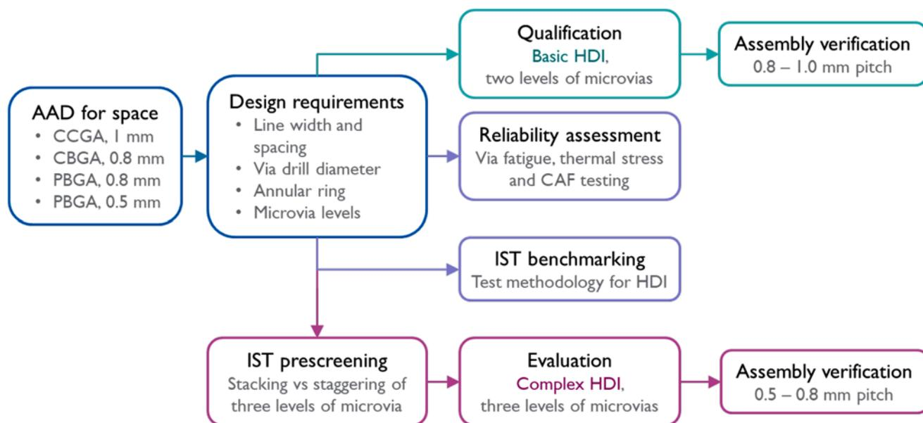
Figure 1: Overall concept for the HDIPCB project.
